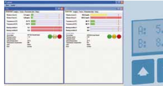
The online display of actual measurements at a PC provides an overview of the condition of the machines.
