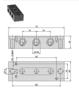
Material: AI (anodized), O-rings: NBR 1 = pressure inlet 3, 5 = exhausts
