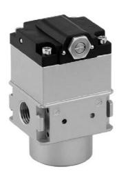
Soft start valve with adjustable filling time. This valve can be used to slowly increase the system pressure through an adjustable throttle. When 50 % of the incoming pressure is achieved the valve opens completely.
