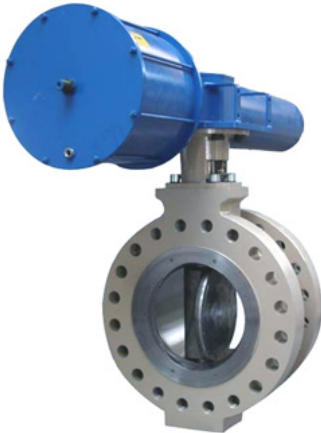
Figure 6.20.1.-8: Leusch Control Butterfly Valve Type LTR 43, triple eccentric, NPS 24 ANSI Class 900 with return actuator
