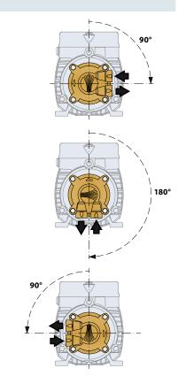
When rotating the pump body it is also necessary to rotate the pump body back-plate
