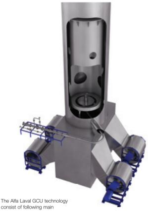
The Alfa Laval GCU technology consist of following main components: exhaust gas stack, combustion chamber including burner, air chamber, combined dilution/combustion fans, gas valve train and control and power panels.
