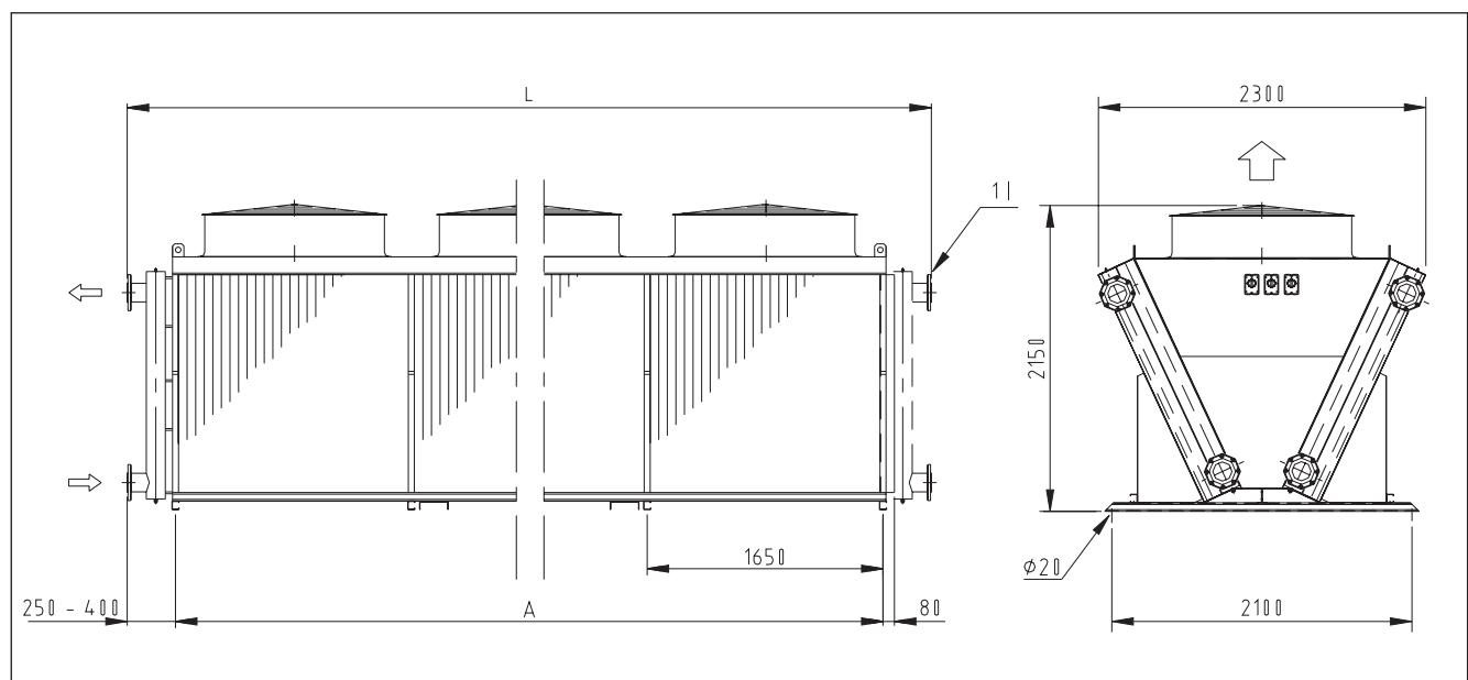
**Condenser tube connection sizes, fan Ø 914 mm PED-classification, 26 bar max. working pressure**
