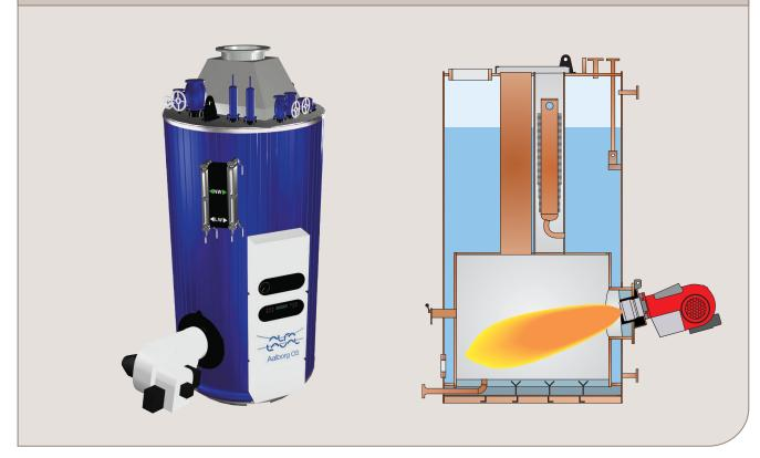
The Aalborg OS is supplied as a standard, preassembled boiler unit. High performance is ensured by the use of the optimally designed pin tube elements. These elements are also used for support of the top plates of the furnace and boiler. The inclined mounting of the burner provides good combustion with all grades.
