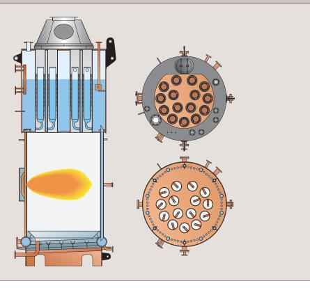
The Aalborg OM boiler is supplied as a standard, pre-assembled unit. The furnace is built of membrane walls with a number of large tubes in between.
