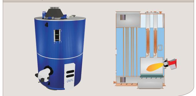
Aalborg OC is a high performance, combined oil and exhaust gas-fired boiler, with a 750-5,000 kg/h capacity of the oil-fired section at 9 bar(g) design pressure. Aalborg OC is a vertical, cylindrical boiler with an exhaust gas section consisting of bare smoke tubes while the oil-fired section features pin tubes in the convection section.
