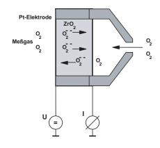
The sensor element consists of a heating coil and a zirconium dioxide disc with electrodes on both sides. The characteristic of  $\rm ZrO_2$  is that it has high conductivity for oxygen ions and poor conductivity for electrons. Because ZrO2 only exhibits this effect substantially at elevated temperatures, a heating coil is used to heat the substrate (heating voltage) to a working temperature of ca. 400°C.
