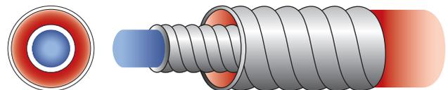
Graphic representation of the flow pattern in the ViscoLine Monotube Unit.
