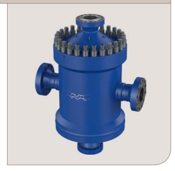
The central distribution tube ensures that the cooling media enters down the middle of the plate, flows around the plate and then exits the other side. Since the nozzles on the shell side are completely independent to those on the plate side the heat exchanger is perfect for asymmetric flow duties.
