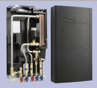
Alfa Laval AquaMicro is a complete, installation-ready district heating substation for domestic hot water. Ilt is suitable for apartments and single family houses that are connected to a heating network. Alfa Laval has long experience in district heating technology and has developed AquaMicro with a well-considered function and simple operation. All components are readily accessible for maintenance and future servicing needs.
